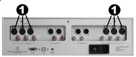
On the rear of the PREAMP 1.0 there are six XLR inputs, three on each side. As you are looking at the rear panel, the left three XLR inputs are for the right channel, the right three inputs are for the left channel. Underneath each jack is the corresponding input number. Use of XLR connections is recommended for the best possible audio quality. To remove an XLR plug, push on the tab above the jack and pull the plug out.
