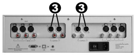
The inner four XLR connections on the rear of the PREAMP 1.0 are outputs. The signal at these outputs is the same—it does not matter if you use output 1 or output 2. To remove an XLR plug, push on the tab on the connector body and pull the plug out.
