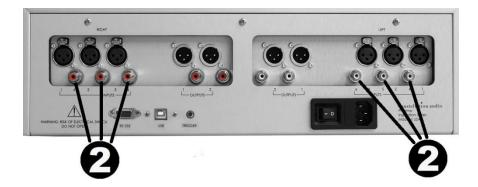
These unbalanced inputs are provided as a convenience for use with unbalanced signal sources. Whenever possible, we recommend using XLR connections instead. Connecting to an unbalanced source is handled in the same way an XLR balanced source.
