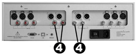
RCA unbalanced outputs are supplied for amps and recording devices not equipped with XLR inputs. The signal at these outputs is the same—it does not matter if you use output 1 or output 2. From left to right, looking at the back of the PREAMP 1.0, the outputs are:  $1_{\text{right}}$ ,  $2_{\text{right}}$ — $2_{\text{left}}$ ,  $1_{\text{left}}$ .
